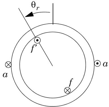
Winding  $a$  has 100 turns and winding  $f$  has 50 turns.  $\mathfrak{R}_m = 2000 \text{ H}^{-1}$ . Neglect leakage inductances and assume variations are sinusoidal.
