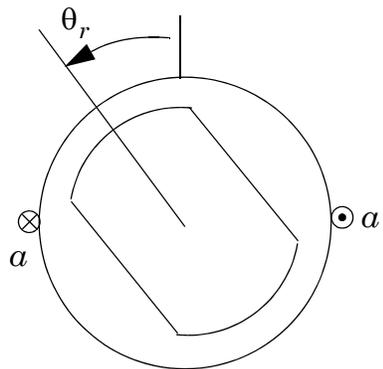
Winding  $a$  has 100 turns.  $\mathfrak{R}_{m, \max} = 1000 \text{ H}^{-1}$ ,  $\mathfrak{R}_{m, \min} = 500 \text{ H}^{-1}$ . Neglect leakage inductance.
