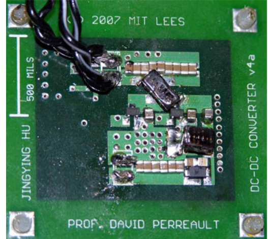
Fig. 14. Photograph of 20 MHz experimental prototype.
