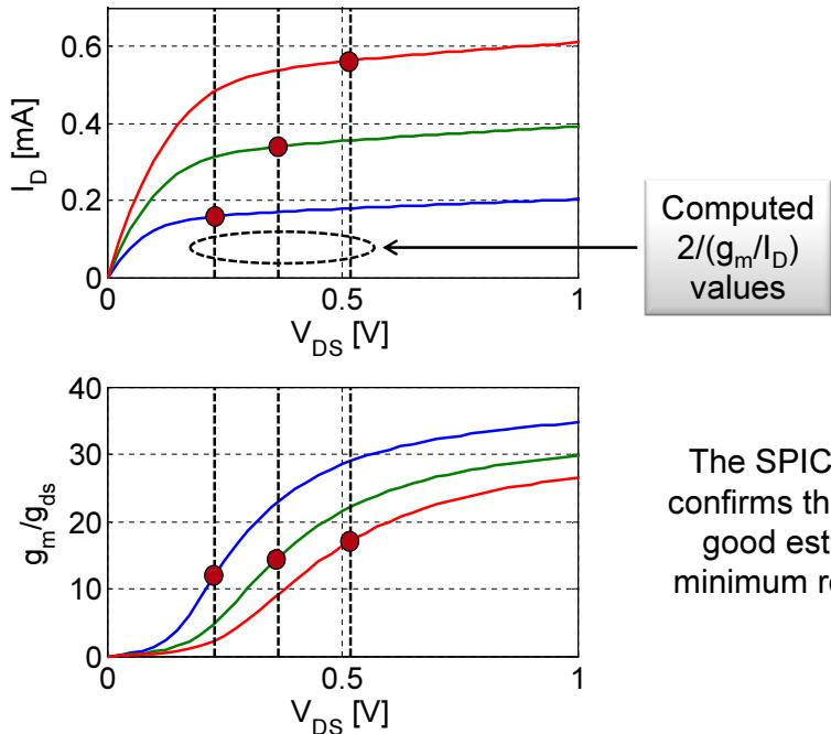
The SPICE model data confirms that  $2/(g_m/I_D)$  is a good estimate for the minimum reasonable  $V_{DS}$
