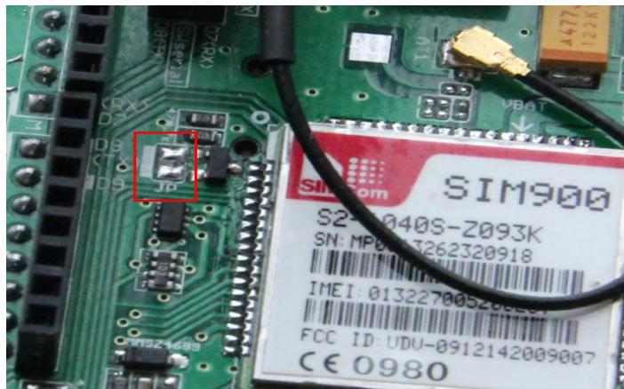
**Software Trigger;** If use this way to power up the GPRS Shield, JP need to be soldered, then Digital Pin 9 of the Arduino will act as Software Trigger port and Digital Pin 9 cannot be use as other purpose. Then give Digital Pin 9 a Turn on Impulse can power up the GPRS Shield. The power up scenarios illustrates as following figure:
