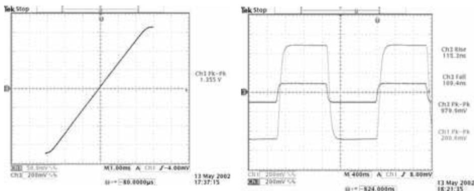
Non-inverting Gain= 5 with 2 internal resistors
