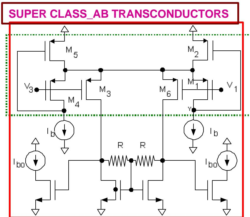
0.5  $\mu$ CMOS,  $V_{DD} = 2$  V,  $C_L = 80\text{pF}$
