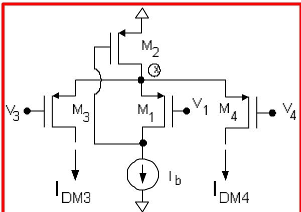
**Symmetrical Class-AB Pseudo Differential Pair (FVF-PDP)**
