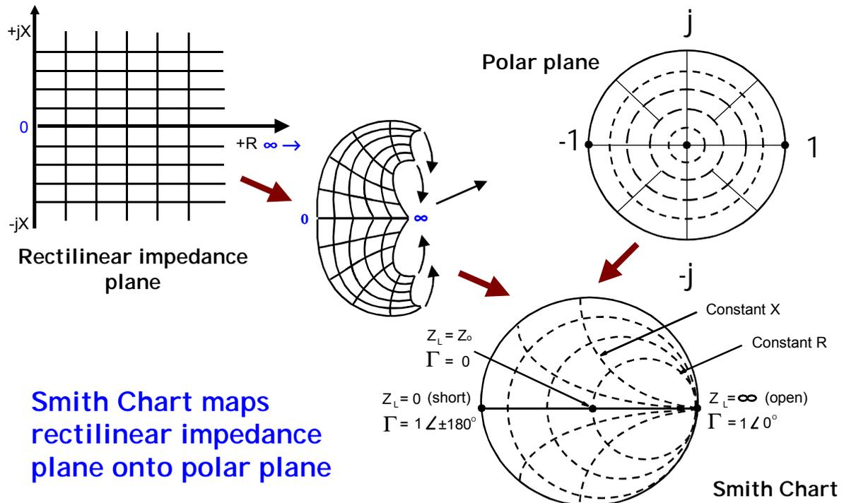
Fig. 3: how the complex resistance plane is transformed into the Smith chart
