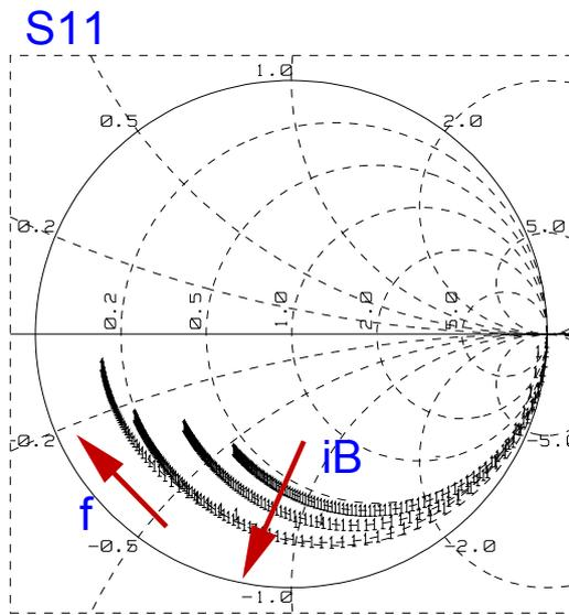
Fig.4a:  $S_{11}$  of a transistor with increasing Base current  $i_B$ .
