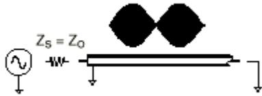
Fig.1: a transmission line connected to a VNA
