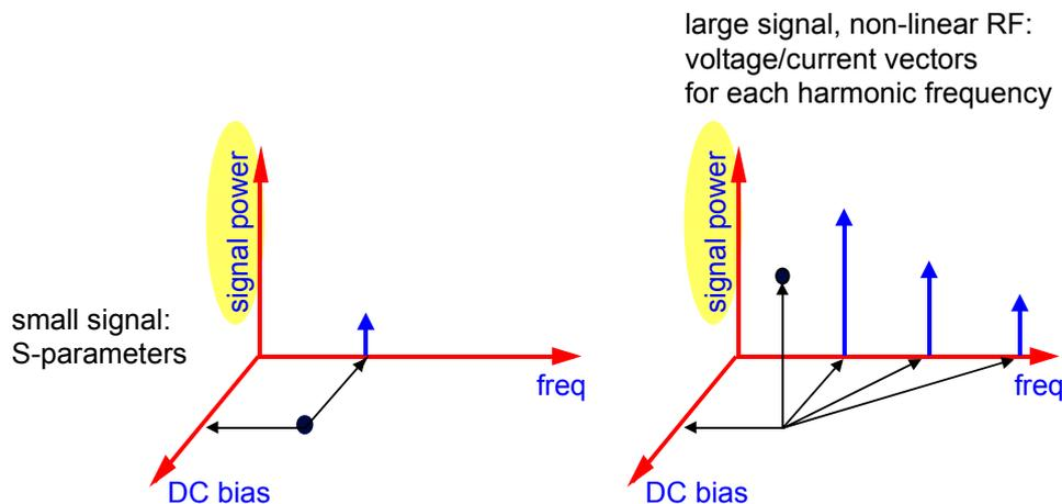
Fig.1: small signal S-parameters are a function of frequency and, for transistors, also of bias, while large signal S-parameters also cover the signal power.
