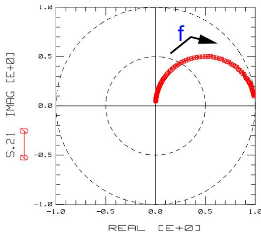
Fig3: S21 of a capacitor between port 1 and port 2
