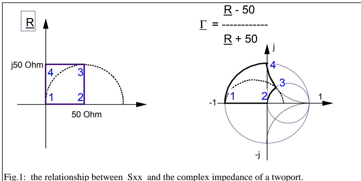
Fig.1: the relationship between  $S_{xx}$  and the complex impedance of a twoport.
