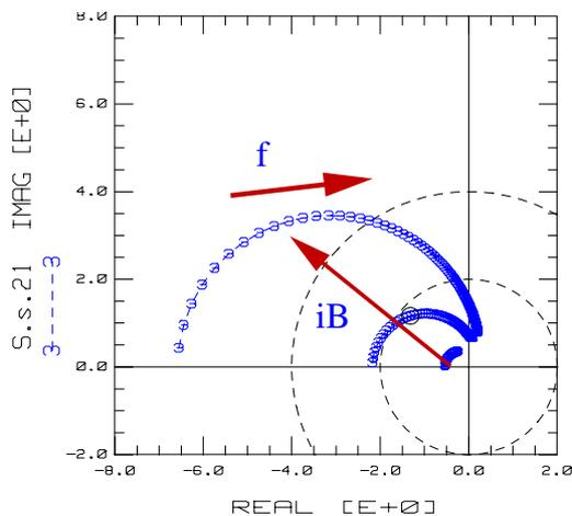
Fig.2: S21 of a transistor with varying Base current  $i_B$ .
