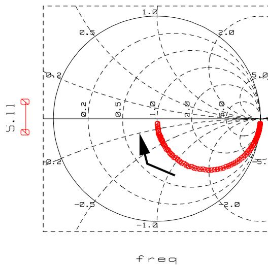
Fig4b:  $S_{11}$  of a capacitor between port 1 and port 2
