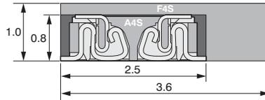
2. **“TOUGH CONTACT ADVANCED”** structure adopted to ensure high resistance to various environments in spite of the ultra-slim and low profile body
