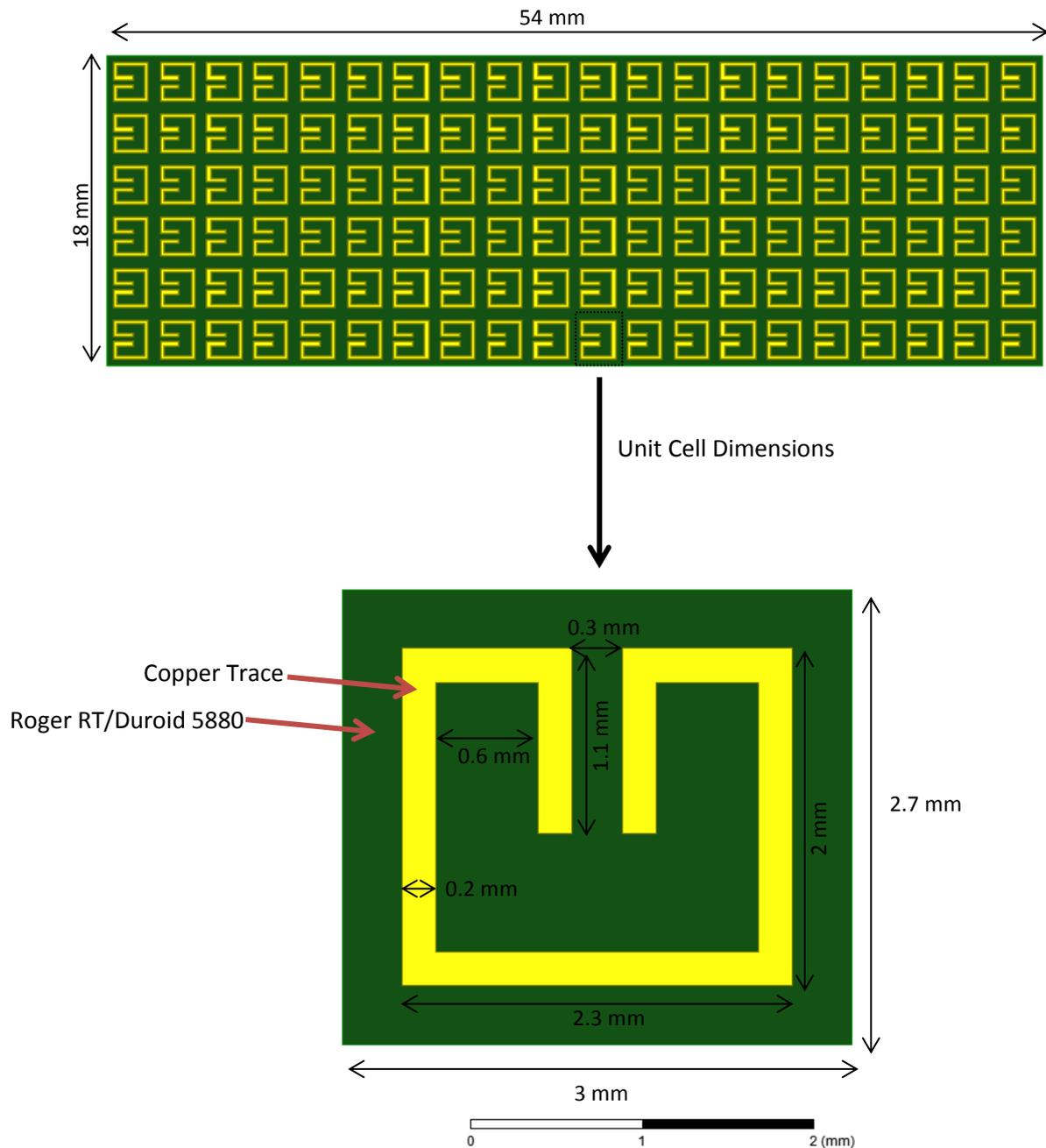
\* Substrate was chosen to be RT/duroid 5880 with ½ oz. (18mm) rolled copper cladding with 0.015”(0.381mm) dielectric thickness.
