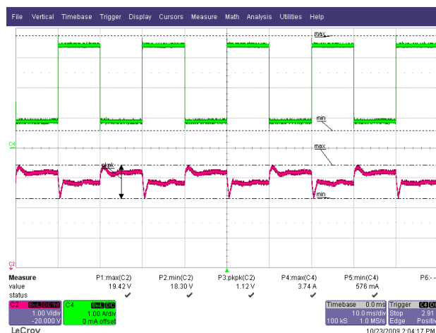
Figure 45 – Transient Response, 90 VAC, 25-100-25% Load Step. Upper: Load Current, 1 A / div. Lower: V_{\text{OUT}} , 1 V / div. Time Scale: 10 ms / div.
