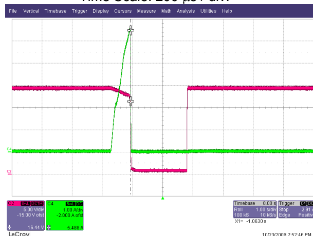
Figure 39 – 230 VAC, OCP Auto Recovery. Upper: I_{OUT} , 1 A / div. Center: V_{OUT} , 5 V / div.
