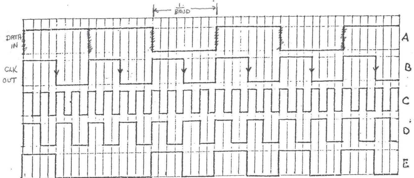
The bandwidth (tracking) is determined by the expression:  $B = 2R/N$  where  $B$  is the bandwidth in hertz,  $R$  is the bit rate in bits/sec, and  $N$  is the basic divide number, or phase increment. The tracking bandwidth is usually symmetric about the center frequency, i.e., the free running frequency with no input applied. Thus a loop for a 3600 BPS data input and a requirement of 10 Hz bandwidth, requires a divide chain of 720 and an oscillator of 5.184 MHz.
