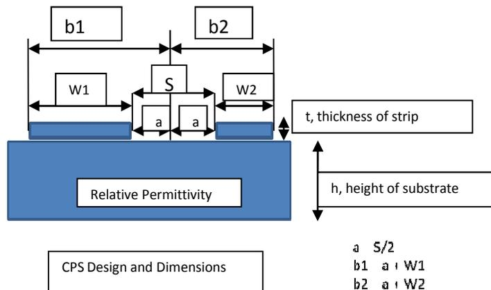
For the equally wide strips,  $b_1 = b_2$
