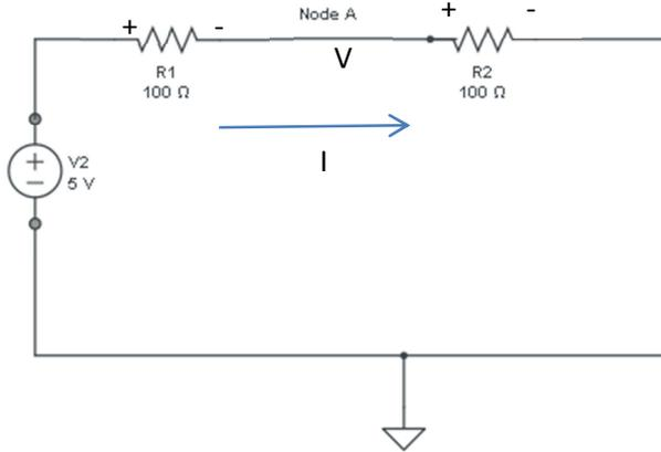
My aim is to calculate the voltage at node A that is voltage V.
