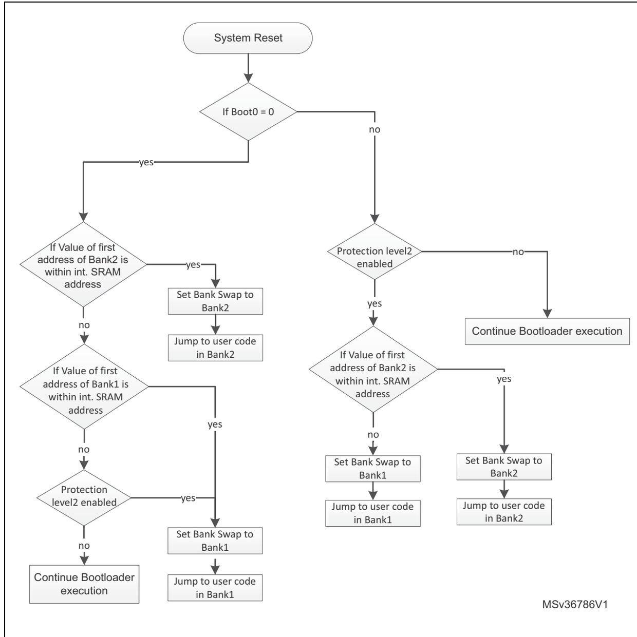
Figure 47.Bootloader V10.x selection for STM32L476xx/486xx
