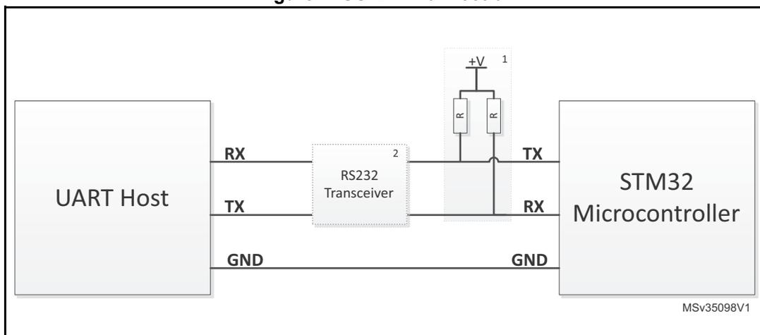
1. A Pull-UP resistor should be added, if pull-up resistor are not connected in host side.
