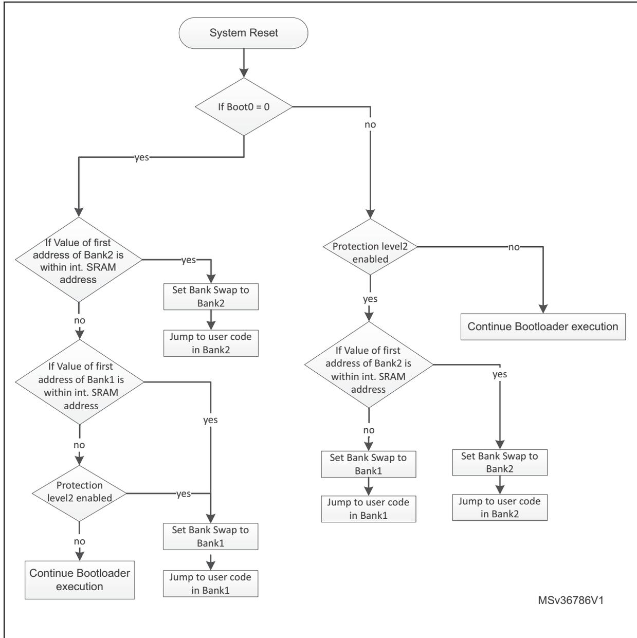
Figure 49.Bootloader V9.x selection for STM32L476xx/486xx
