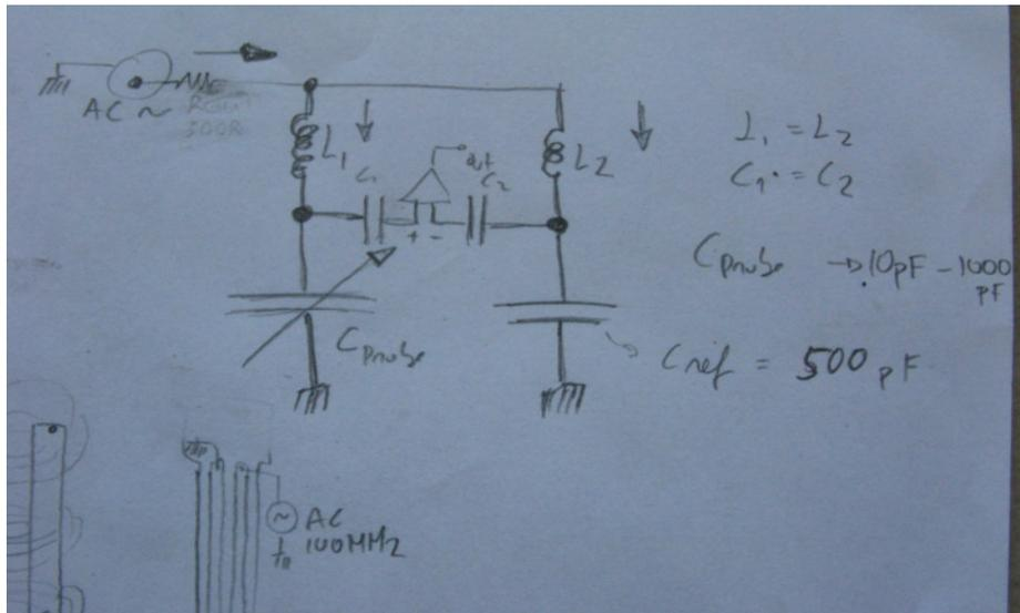
Wheatstone bridge with AC in from LTC6905 100MHz 3Vpp (datasheets says 3Vpp 500ohm load)
