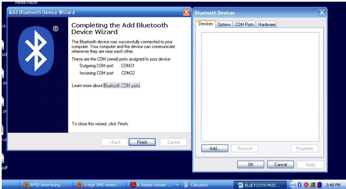
We can see the COM ports assigned to the Bluetooth dongle as COM 21 as Outgoing and COM22 as Incoming.
