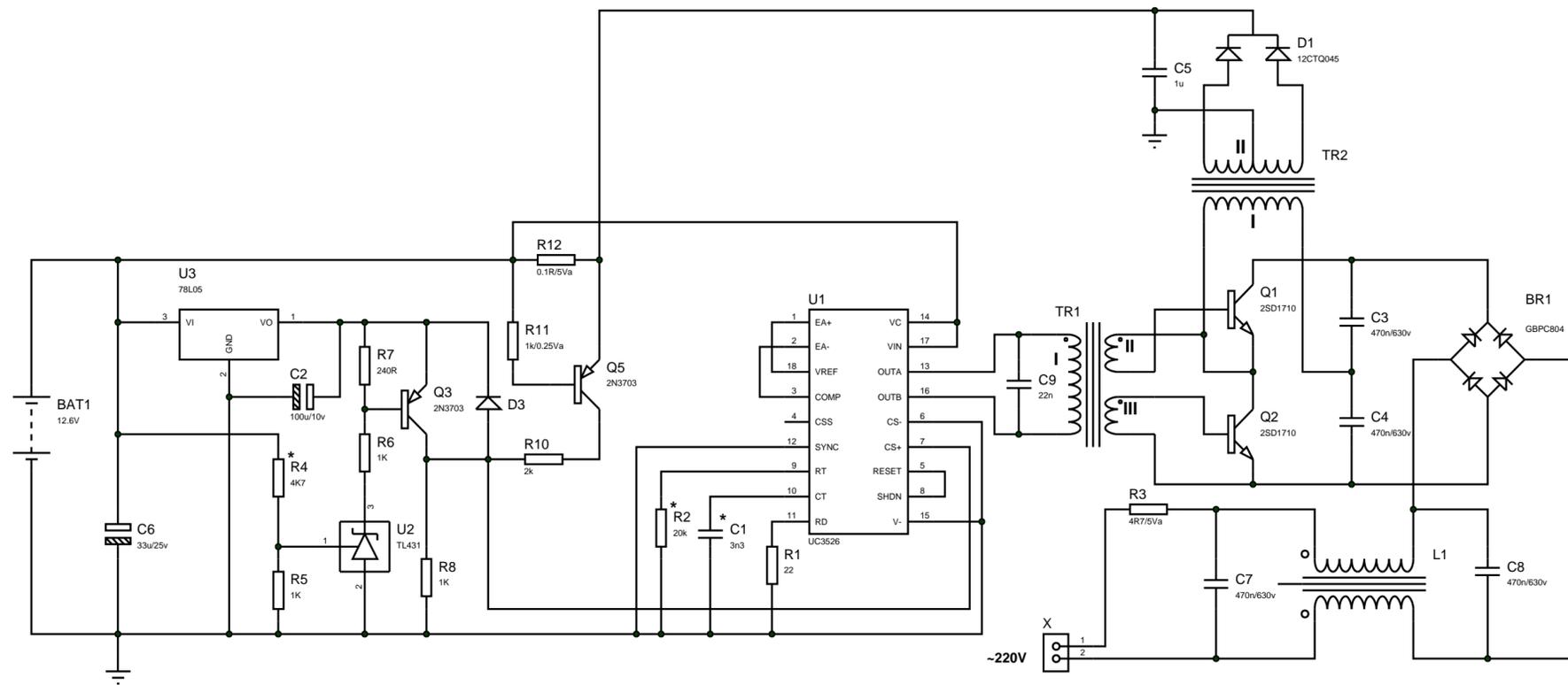
Initial power supply of the generator on chip U1 is carried out from the charged battery through a surge protector on chip U3, therefore inclusion in a device network will not lead to the inverter start, the consumed current is practically equal to zero.
