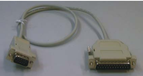
Fig.1 ISP CABLE :12NC IS "3138 106 10148".
