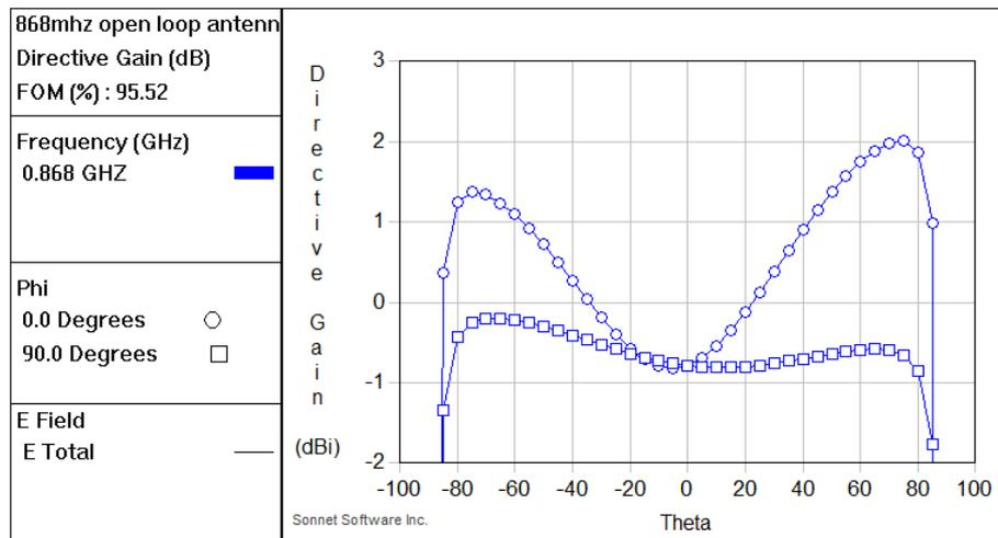
Due to the simulation method with a substrate that extends to infinity, the value at the horizon (Theta= $\pm 90^\circ$ ) is not exact. The drop seen in the simulation is a simulation artefact and does not exist in reality.
