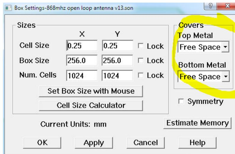
Technically, this setting places absorbing boundaries at the top and the bottom of the simulation box.
