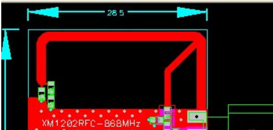
The planar antenna consists of an "n"-shaped PCB trace that is tapped by a feed line at a well defined position. One end of the trace is directly connected to the reference metallization (lower right hand side in the picture), and the other end is connected via a set of SMD elements to the reference metallization (lower left hand side).
