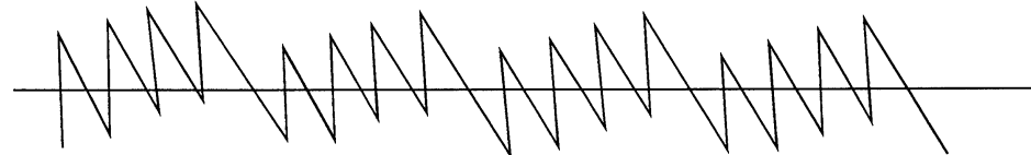
Figure 3.133: Idling Patterns for First-Order Sigma-Delta Modulator (Integrator Output)
