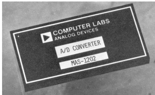
MAS-1202 12-BIT, 2 \mu s SAR ADC INTRODUCED IN 1975
