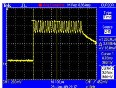
The Midea IR signal uses pulse distance encoding. Each pulse (one "time" unit or 1T) is 21 cycles of a 38KHz carrier burst (about 550 $\mu$ s long). A logic "1" is a 1T pulse followed by a 3T space and takes 2.25ms to transmit. A logic "0" is a 1T pulse followed by a 1T space and takes 1.125ms. The AGC burst consists of a 4.5ms burst followed by 4.5ms space (8T pulse + 8T space). This is very close to the RCA infrared standard.
