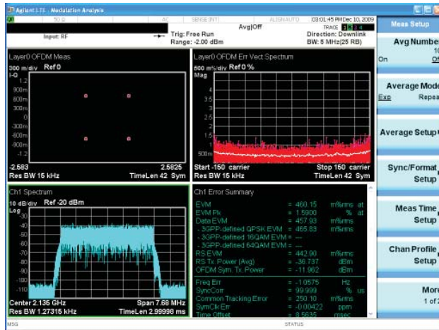
Figure 7c. 5 MHz E-TM 1.1 signal with baseband filter and symbol rolloff length = 20 T_s .
