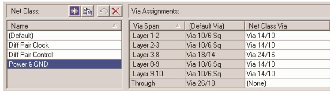
The screenshot shows a dialog box with two main sections: 'Net Class:' and 'Via Assignments:'. The 'Net Class:' section has a list of net classes with 'Power & GND' selected. The 'Via Assignments:' section is a table with three columns: 'Via Span', '(Default Via)', and 'Net Class Via'.
