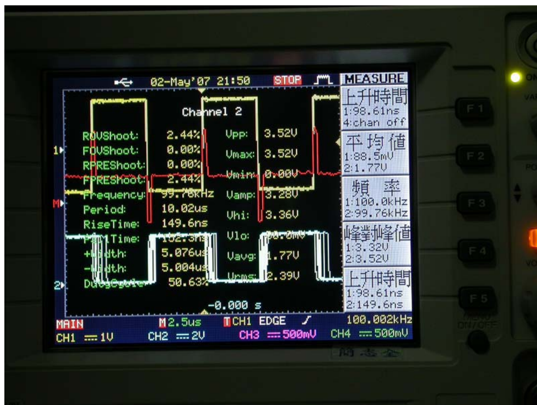
Fig. 12 A typical oscilloscope output for ADPLL
