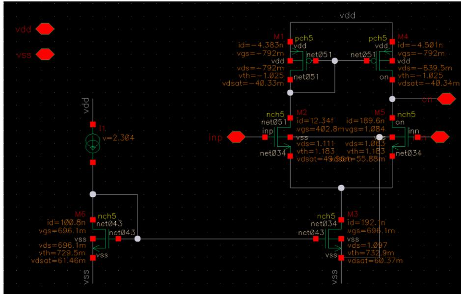
And the 1-bit DAC that is used in the loop is:
