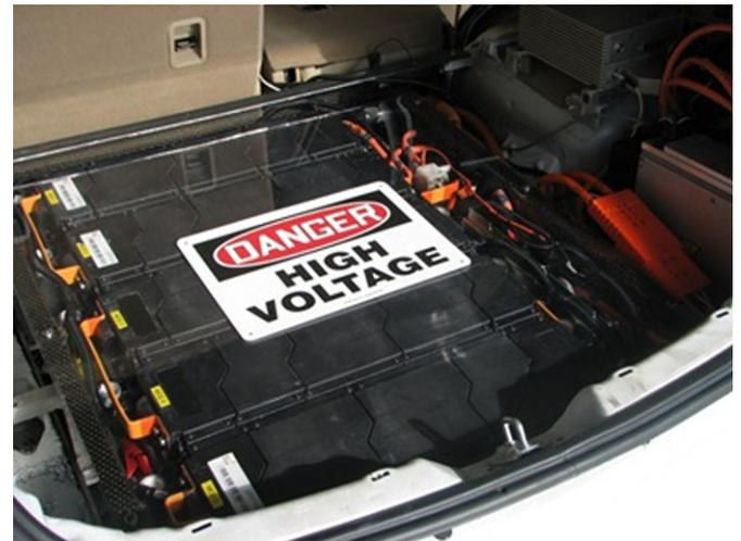
Fig. 16. The A123 lithium-ion battery pack installed in the Mississippi State University EcoCAR.
