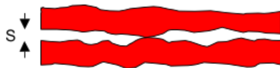
Fig 3.2: Short between two excessively close poly lines.
