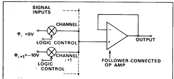
Figure 2. Simplified diagram of multiplexer circuit
