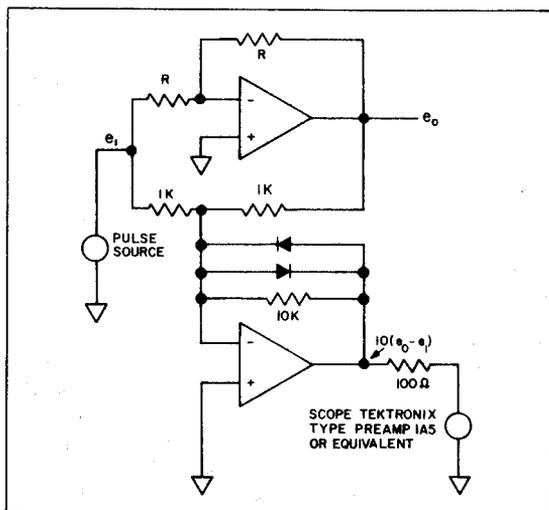
Figure 10. Settling Time Measurements at Quasi-Summing Point.
