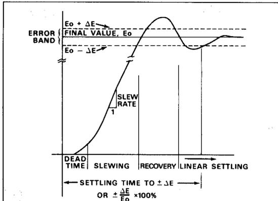
(a) Components of settling time (nonlinear scale)
