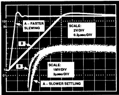
(b) Annotated wave forms illustrating comparative settling time of two typical op amps.
