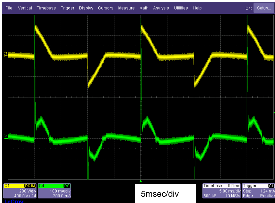
Figure14. Dimming operation waveform at phase angle=60degree
