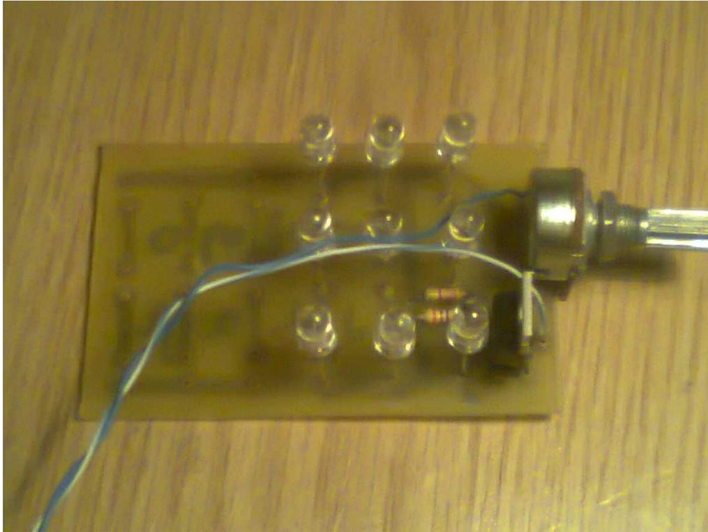
18 white led's were included on the pcb, but I used only 9. I remarked that better dispersion of the led's on the board will improve the the efficiency, so I suggest a 1 inch distance between led's
