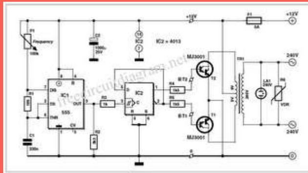
As the output current available from the CMOS 4013 is very small, Darlington power transistors are used to arrive at the necessary output current. We have chosen MJ3001s from the now defunct Motorola (only as a semi-conductor manufacturer, of course!) which are cheap and readily available, but any equivalent powerDarlington could be used.
