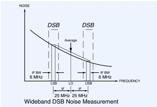
In the wideband DSB receiver architecture, the IF is 25 MHz and the bandwidth is 6 MHz. The frequency measurement range is comprised of 12 MHz of frequency separated by 44 MHz, or 56 MHz (12 + 44 MHz). As expected, this architecture can be more susceptible to DUT noise figure variations than the SSB architecture, which only used 4 MHz. This comparison indicates more measurement uncertainty can be associated with the wideband DSB receiver architecture than the SSB receiver architecture.
