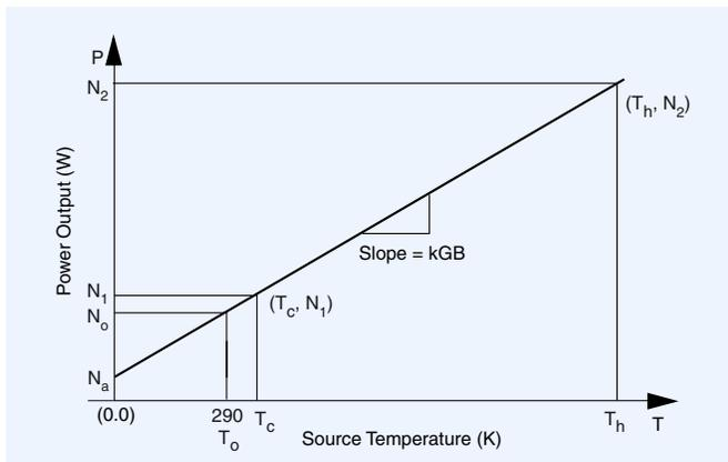
The terms  $T_{on}$  and  $T_{off}$  are sometimes substituted for  $T_h$  and  $T_c$ . The noise power associated with  $T_h$  is labeled  $N_2$  and the noise power associated with  $T_c$  is labeled  $N_1$ . The ratio of  $N_2/N_1$  is the Y-Factor. Using ordinary algebra, these two points determine the noise power ratio and the noise figure for the measurement.
