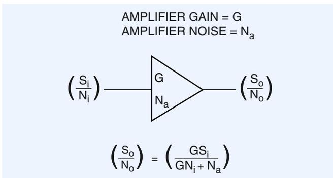
Clearly, the input signal power,  $S_i$ , and the input noise power,  $N_i$ , increase by a factor of  $G$  when passing through an amplifier. Less clear is that the shot and thermal noise generated within the amplifier,  $N_a$ , adds to the output noise power,  $N_o$ . In this case,  $N_o$  is the combination of  $GN_i$  and  $N_a$ . Indeed, the resulting output signal-to-noise ratio degrades from the input signal-to-noise ratio by the addition of this inherent amplifier noise power,  $N_a$ .
