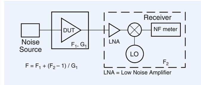
Solving this equation for  $F_1$  allows the instrument to calculate the DUT noise figure from the overall cascaded noise figure measurement. The following equation shows the results after solving for  $F_1$ .
