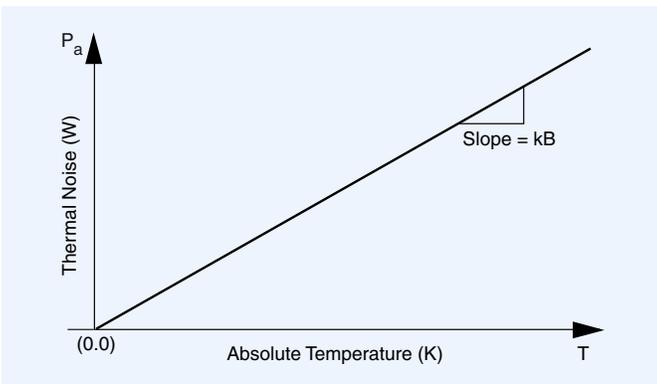
In this graph, the Y-axis indicates noise power and the X-axis indicates the absolute temperature. It is significant to note that the slope of this output is  $kB$  and that an absolute temperature of  $0K$  produces thermal noise of zero Watts. This zero crossing also describes a Y-axis intercept. Incorporating this slope and this Y-axis intercept into the equation for a line yields the following equation for thermal noise.
