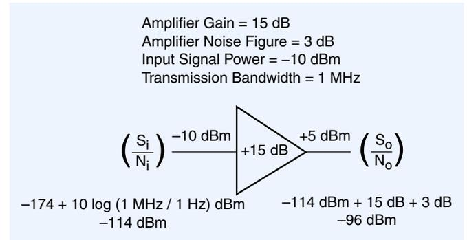
The following table verifies the noise figure of 3 dB by applying both noise figure definitions to this amplifier under the given conditions. The values in Watts have been converted from the corresponding values in dBm.
