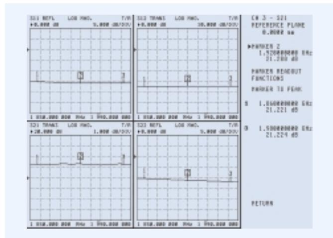
Note that the input matching is greater than 15 dB and the output matching is greater than 10 dB. The scalar and vector error-corrected noise figure measurements should produce similar results based on this matching performance.
