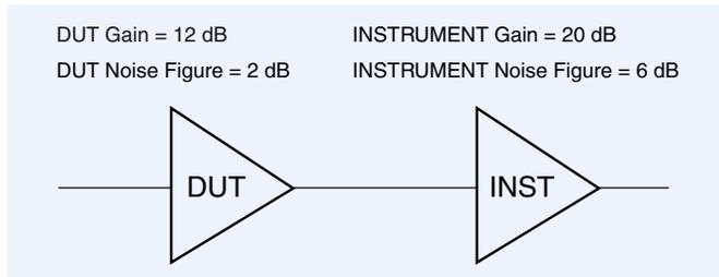
The cascaded noise figure equation is in linear terms; therefore, convert the noise figure and gain from the logarithmic to the linear form. Perform all the calculations in linear terms and convert to logarithmic for the final results. The following conversion equations indicate the relationship between the logarithmic and linear terms.
