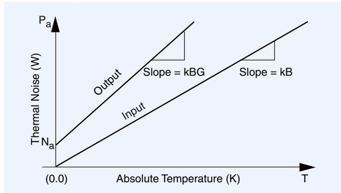
The noise power output characteristics are the product of the amplifier gain and  $kTB$ , or  $kTBG$ . The slope of this noise power output is  $kBG$ ; furthermore, the noise power output for absolute temperature of zero is the added noise power,  $N_a$ , generated within the amplifier. This observation leads to a straightforward technique for measuring the added noise power generated within the amplifier.
