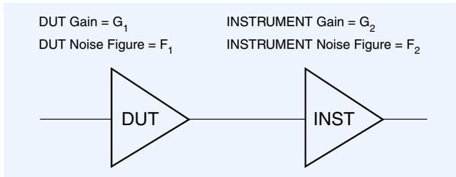
The DUT has available gain of  $G_1$  and noise figure of  $F_1$ . Similarly, the instrument has gain of  $G_2$  and noise figure of  $F_2$ , typically acquired during calibration. The following equation yields the overall noise figure ( $F$ ) for this cascaded network.
