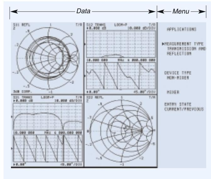
Notice that the display is partitioned into the data and the menu display areas separated by a vertical line. The menu display area provides the selection mechanism for the MS462xx and will be the focus of this section.
