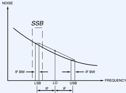
Spectrum of SSB Noise Measurement
