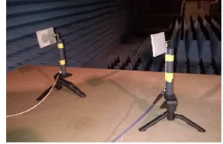
Fig. 6. Free space fidelity ( S_{12} ) measurement setup in an anechoic chamber.
