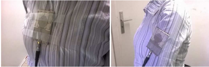
Fig. 4. OSUA on-body measurement setup with the antenna placed on the chest and on the arm, respectively.
