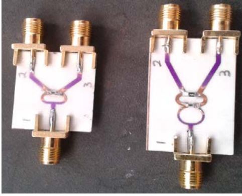
Fig. 5. Photograph of the fabricated single and double stage Wilkinson power divider.
