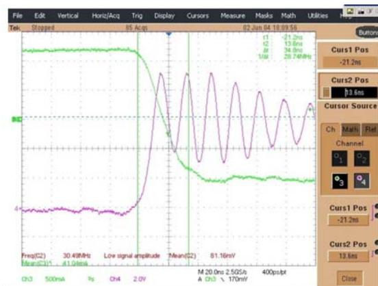
**FIGURE 9.** Measured current and voltage turn-off switching transient.
