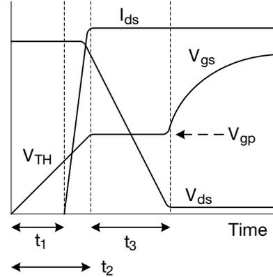
Fig. 2 - Turn-On Transient of the MOSFET
