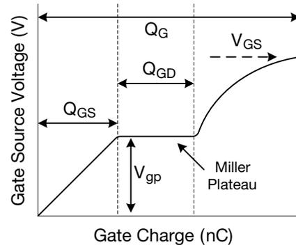
Fig. 4 - Sketch Showing Breakdown of Gate Charge
