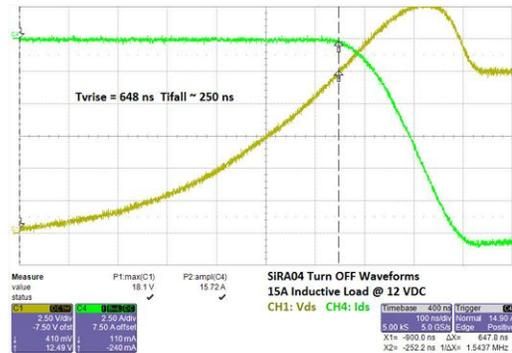
Fig. 7 - Measured Current and Voltage Turn-Off Switching Transient
