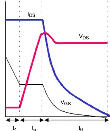
**FIGURE 5.** Turn-off transient of the MOSFET.
