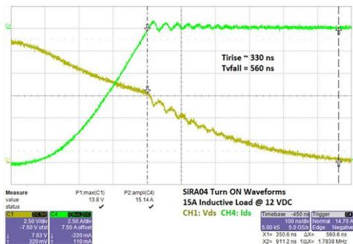
Fig. 6 - Measured Current and Voltage Turn-On Switching Transient
