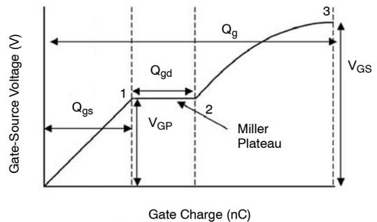
**FIGURE 6.** Sketch showing breakdown of gate charge.
