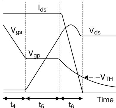
Fig. 3 - Turn-Off Transient of the MOSFET
