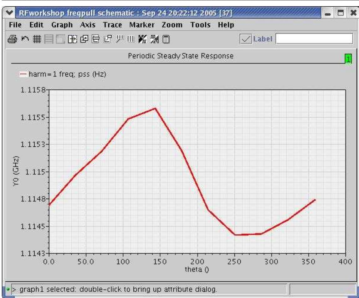
The peak to peak difference in the displayed frequency in the above figure gives the load pull.
