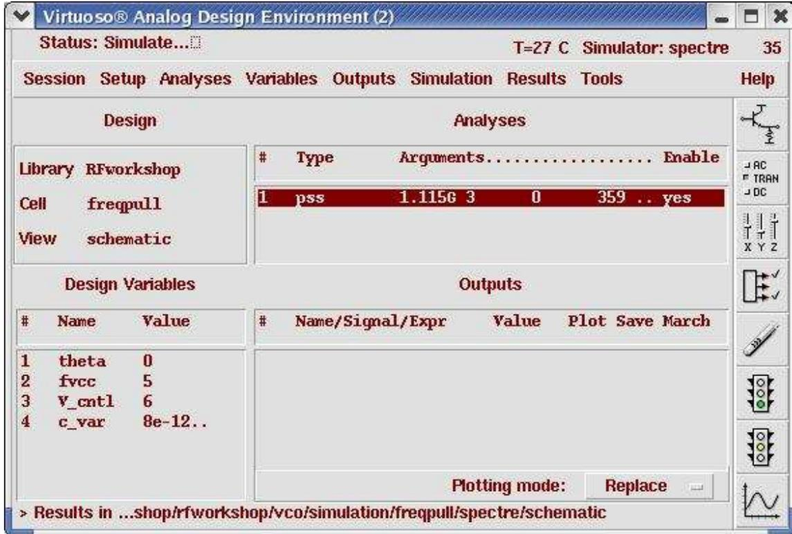
**Action5-8:** In your Analog Design Environment, Choose **Simulation—Netlist and Run** or click the **Netlist and Run** icon to start the simulation.
