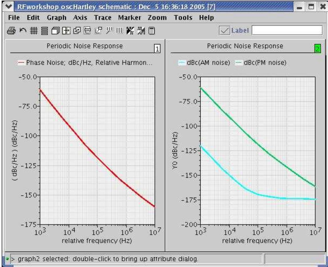
**Action1-24:** Compare the total phase noise to the PM noise. Move your mouse cursor in the waveform window and read the phase noise plot and the PM noise at 10K Hz. They are the same.
