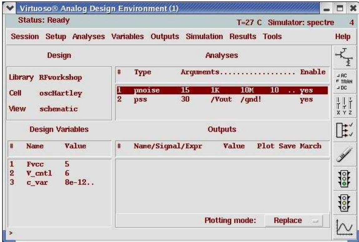
**Action1-35:** In your Analog Design Environment, Choose **Simulation—Netlist and Run** or click the **Netlist and Run** icon to start the simulation.
