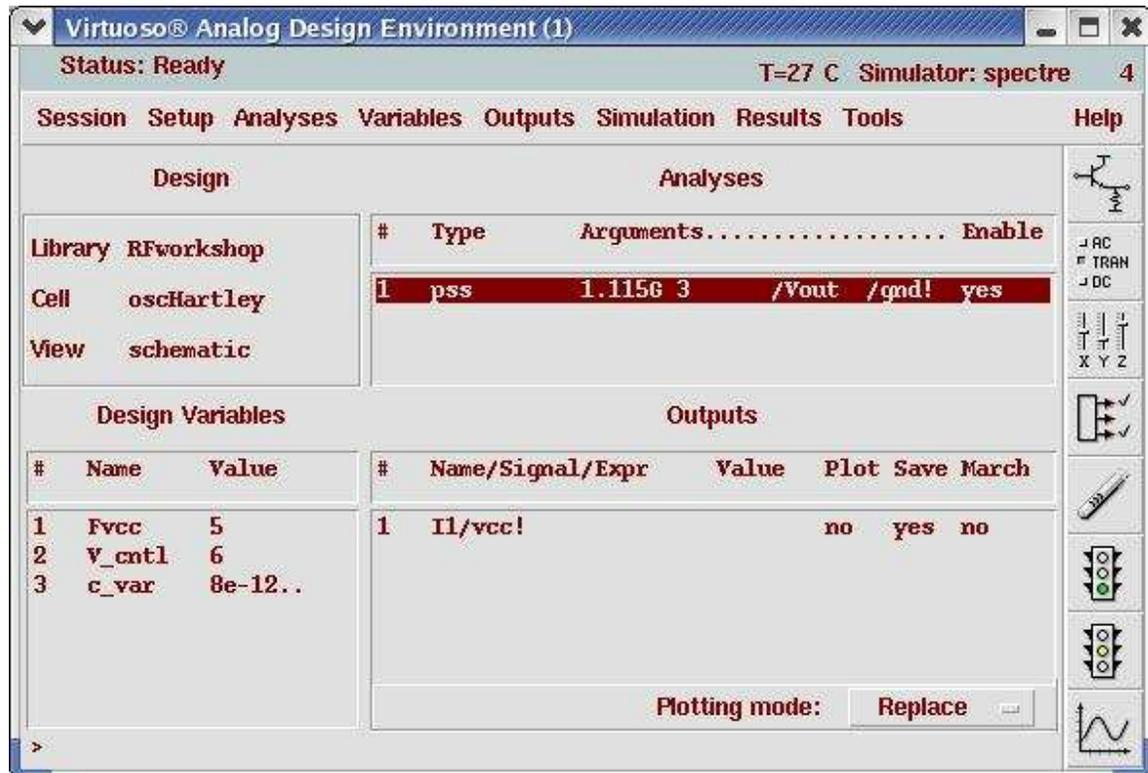
**Action4-11:** In your Analog Design Environment, Choose **Simulation—Netlist and Run** or click the **Netlist and Run** icon to start the simulation.
