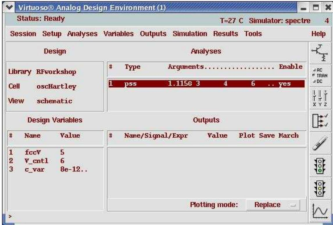
**Action2-8:** In your Analog Design Environment, Choose **Simulation—Netlist and Run** or click the **Netlist and Run** icon to start the simulation.
