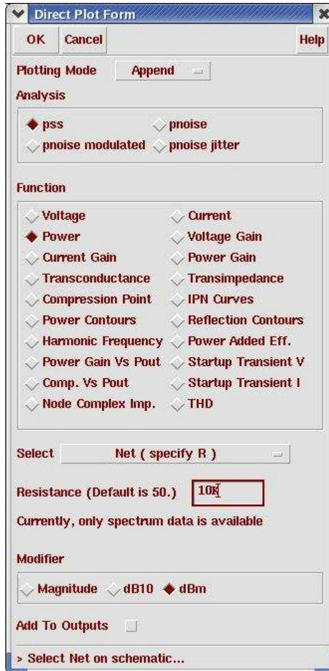
**Action1-19:** Select net Vout on the schematic. The results show the oscillation frequency is around 1.1G, and output power is around 0 dBm.
