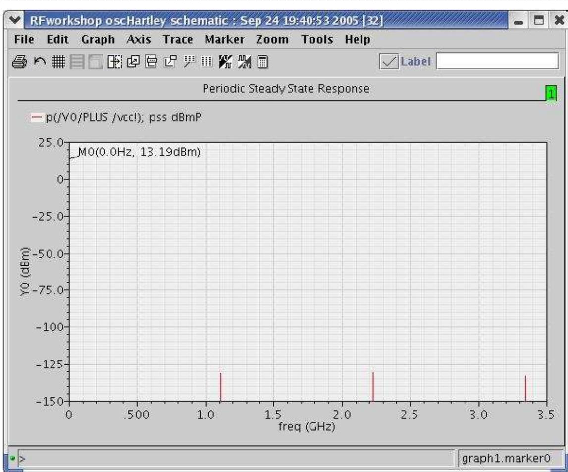
Power dissipation is the value that corresponds to the DC value in the above figure; that is, at freq = 0.0 the power dissipation value is equal to -16.81 dB or 13.19 dBm.
