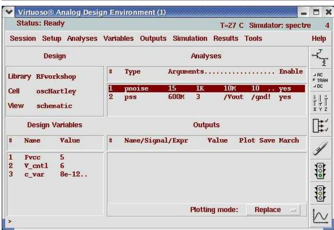
**Action1-12:** Choose **Simulation—Netlist and Run** to start the simulation or click on the **netlist and Run** icon in the Virtuoso Analog Design Environment window.
