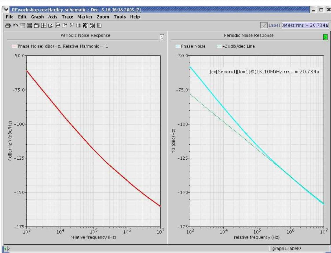
MMSIM60USR2 introduces Flexible Balance for autonomous circuit application. In this release FlexBalance is supported for oscillators and phase-noise simulation. Flexbalance is a frequency domain technique similar to Harmonic balance which solves the spectra of each node voltage unlike the time-domain technique (such as shooting PSS) which solves the waveform of each node voltage over the period.
