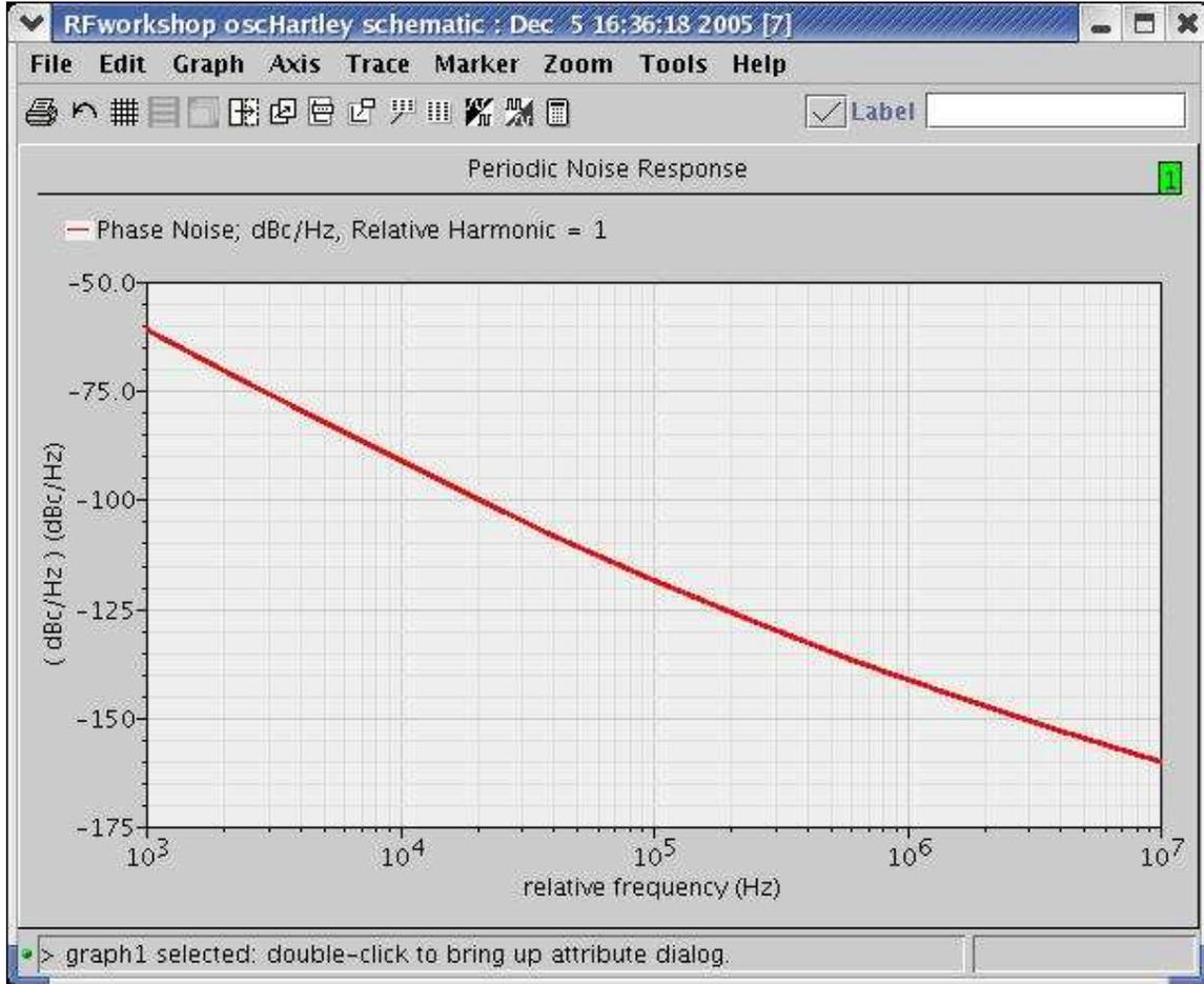
SpectreRF determines autonomous Jitter by first determining noise versus frequency with correlations (modulated Pnoise). When running pnoise modulated, SpectreRF compute correlation between sidebands by using pnoise=correlation in the background. Using spectreRF Pnoise modulated analysis, the user can fully characterize AM, PM, USB and LSB components of the noise.
