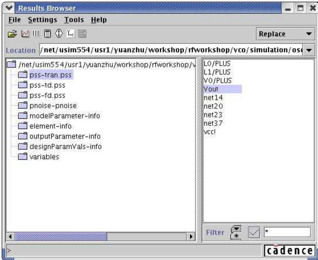
**Action1-15:** Double click on Vout. The *Vout* transient node voltage appears in the Waveform window.
