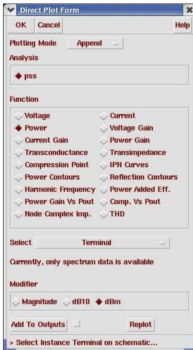
**Action4-14:** Click the positive terminal of pulse source on the schematic. . The following plot will show up.
