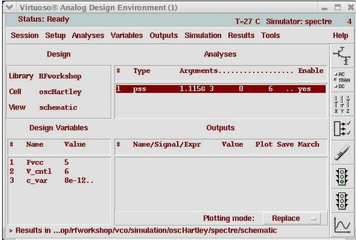
**Action3-8:** In your Analog Design Environment, Choose **Simulation—Netlist and Run** or click the **Netlist and Run** icon to start the simulation.
