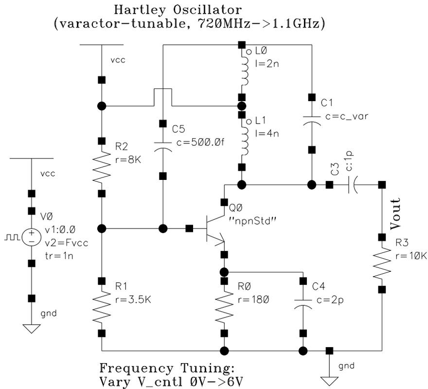
The oscHartley VCO uses the basic Hartley topology and is tunable between 720 MHz and 1.1 GHz. The oscillation frequency ( $F_o$ ) is determined by the resonant circuit made up of inductors ( $L_0$ ,  $L_1$ ) and the  $C_1$  capacitor. In this particular VCO, the values of  $L_1$  and  $L_2$  are fixed whereas the value of  $C_1$  is variable.
