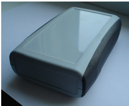
Figure 1 – Enclosure used to accommodate the hardware main board (including the USB sub-board) and the ZIF socket board (PACTEC Model 87836-510-508, PPLX Kit, Grey w/ Black Sides, external dimensions 121.9 x 78.7 x 33 mm).
