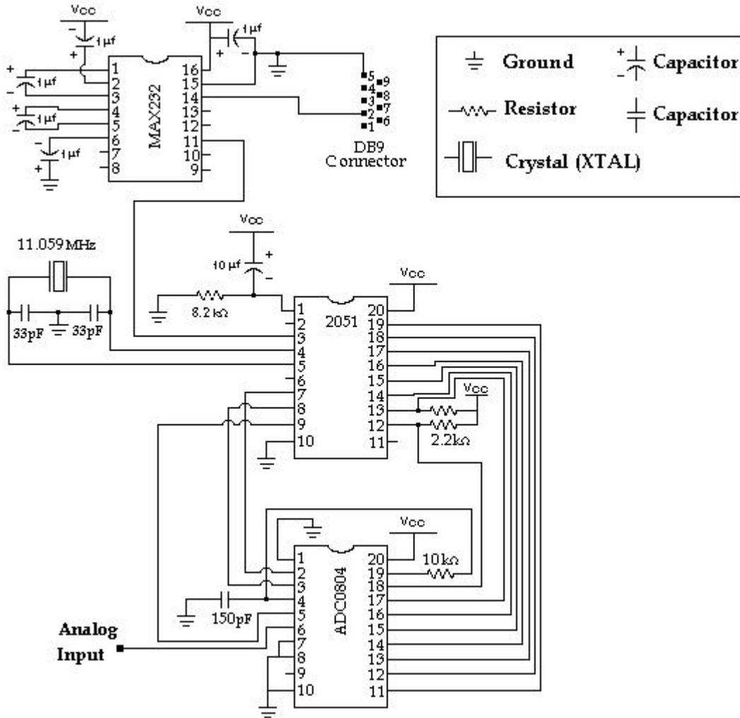
The above circuit explains both the concepts of interfacing an ADC as well as sending the acquired data to the PC through the PC's Serial Port (DB 9). It uses an ADC0804 chip to convert from analog to digital, an AT89C2051 microcontroller to control the ADC0804 and send data to the PC, and a MAX232CPE chip to convert the signals from and to RS232 levels for sending and receiving from the PC.
