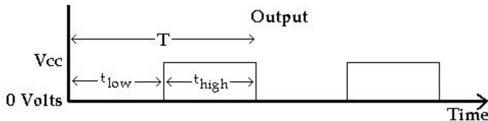
We will always keep  $T$  the same so that there is always the same number of output cycles per second. If we increase the width of  $t_{high}$  then we must decrease  $t_{low}$  to keep  $T$  the same. If we decrease  $t_{high}$  then we must increase  $t_{low}$ . For the case that we make  $t_{high}$  small then the output looks like the following.
