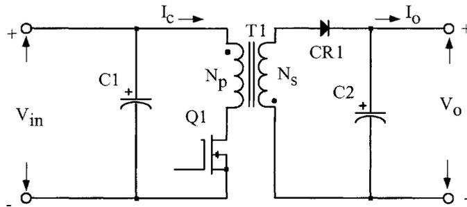
Figure 13-12. Schematic of an Isolated, Buck-Boost Switching Converter.
