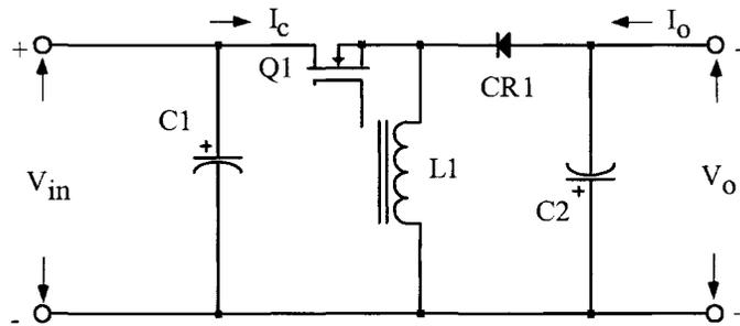
Figure 13-9. Schematic of an Inverting Buck-Boost Switching Converter.
