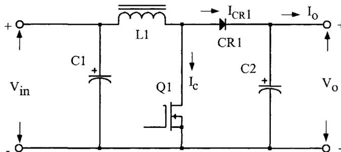
**Figure 13-6.** Schematic of a Boost Switching Converter.
