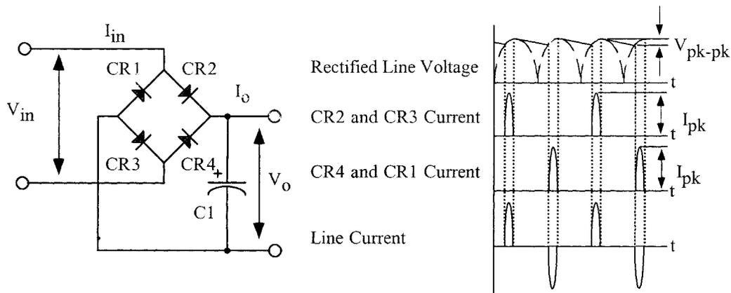
**Figure 13-15.** Typical, Capacitor Input Bridge Rectifier Filter.
