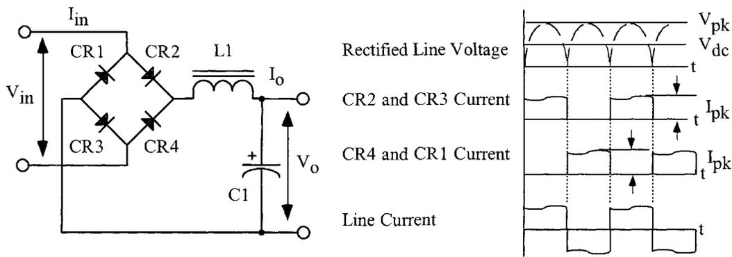
Figure 13-16. A Typical, Inductor Input Bridge Rectifier Filter.
