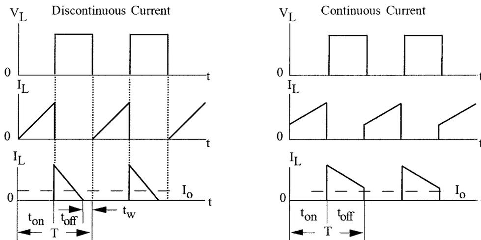
**Figure 13-1.** Comparing Discontinuous and Continuous Current Waveforms.
