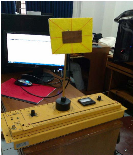
Figure 13: Microstrip Patch Antenna for 2.4 GHz
