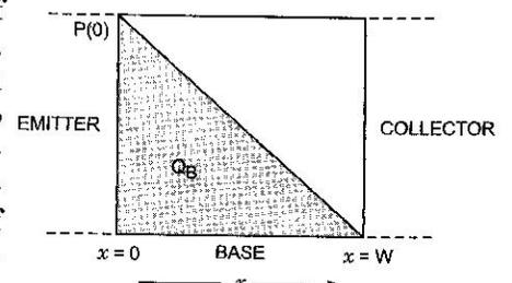
Fig. 14.4. Minority-Carrier Charge Distribution in Base Region
