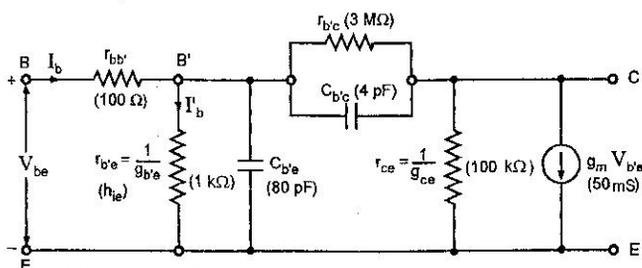
Fig. 14.9. Giacoletto or Hybrid- $\pi$  Model of a Transistor in CE Configuration
