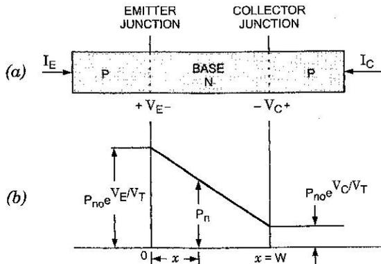
Fig. 14.5. Minority-Carrier Density in The Base Region
