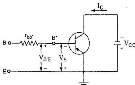
Fig. 14.10. P-N-P Transistor in CE Configuration For The Derivation of Transconductance ( $g_m$ )
