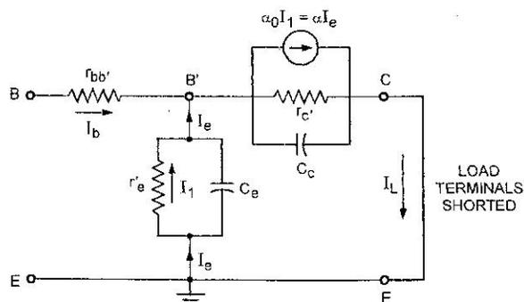
Fig. 14.6. The T-Circuit in The CE Configuration Under Short-Circuit Conditions
