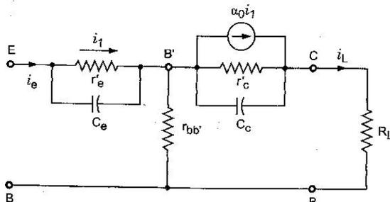
Fig. 14.3. Approximate CB High-Frequency T-Model
