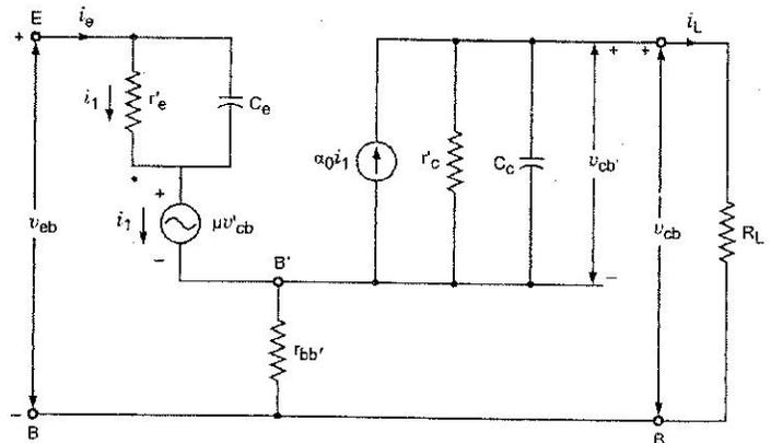
Fig. 14.1. High-Frequency Transistor T Model
