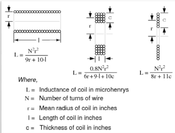
The inductance of multilayer air cored inductor can be calculated using the formula as given in the diagram. For typical 3 milli-henry inductance, 330 Turns of 19 SWG enameled copper wire wound over a bobbin of 1 inch diameter and 1 inch length.
