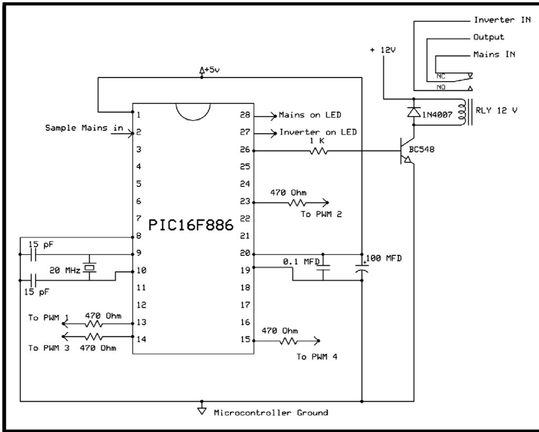
Program written in assembly language for PIC16F886 microcontroller is given below which is fully tested. The HEX file generated for the assembly program is also given at the end of this document. The HEX file may be directly loaded into PIC16F886. The program can be modified to add features such as low battery cutoff, over load protection, Short circuit protection, and High heat sink temperature protection by using LM35 sensor.
