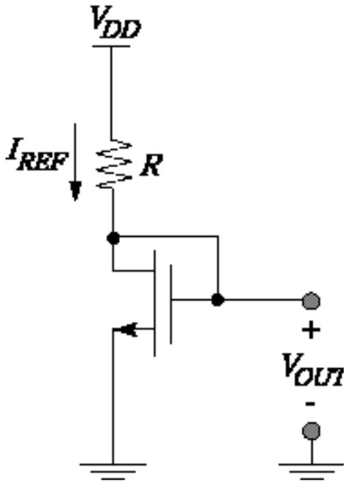
$$I_{REF} = \frac{V_{DD} - V_{OUT}}{R}$$
