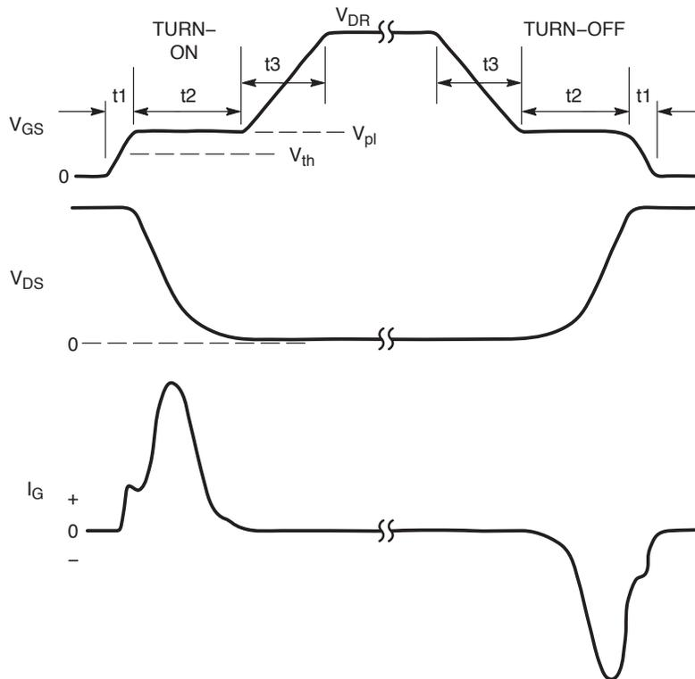
Figure 18. Typical MOSFET Drive Waveforms (Top:  $V_{GS}$ , Middle:  $V_{DG}$ , Bottom:  $I_G$ )
