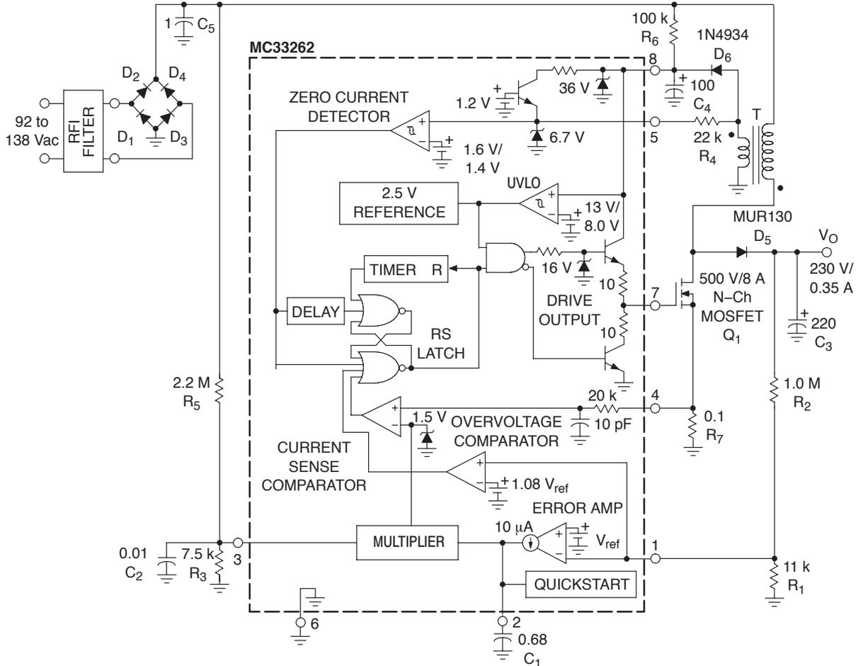
**Figure 42. 80 W Power Factor Controller**
