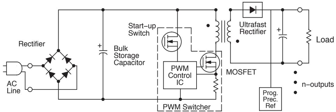
Figure 38. AC/DC Power Supply for CRT Displays
