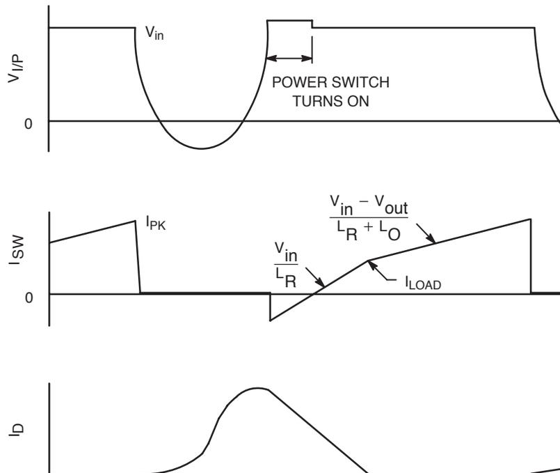
**Figure 32. Schematic and Waveforms for a ZVS Quasi-Resonant Buck Converter**
