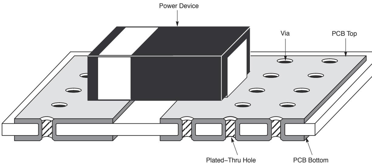
Figure 22. Method for Minimizing AC Capacitive Coupling and Enhancing Heatsinking
