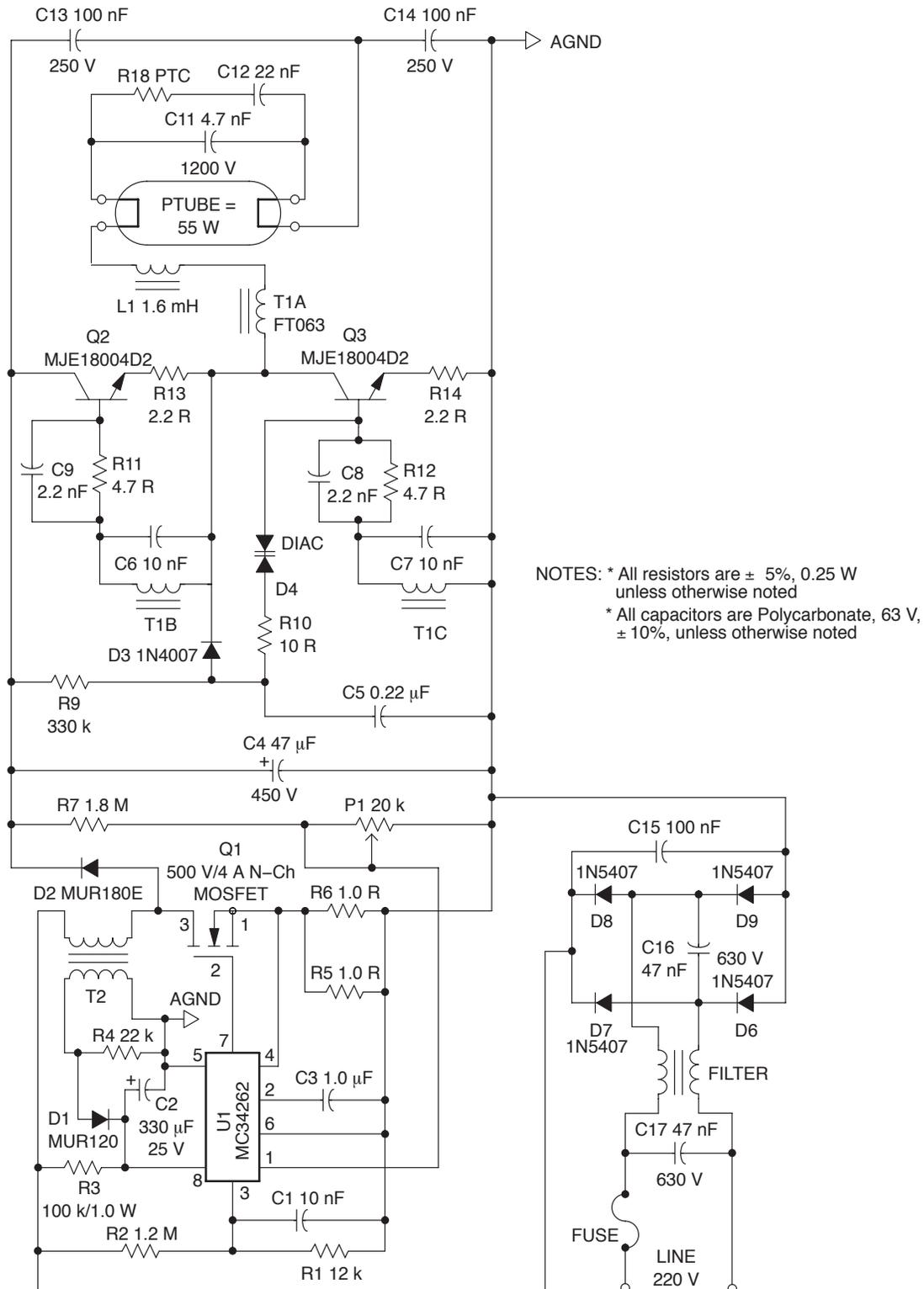
Figure 49. Efficient Safety Circuit for Electronic Ballast
