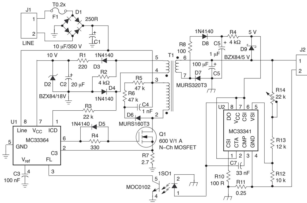
Figure 50. AC-DC Battery Charger – Constant Current with Voltage Limit
