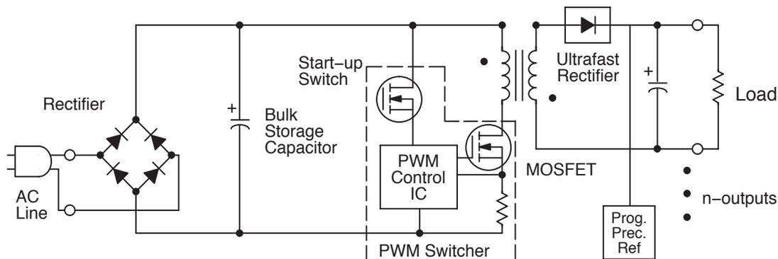
Figure 39. AC/DC Power Supply for Storage, Imaging & Entertainment
