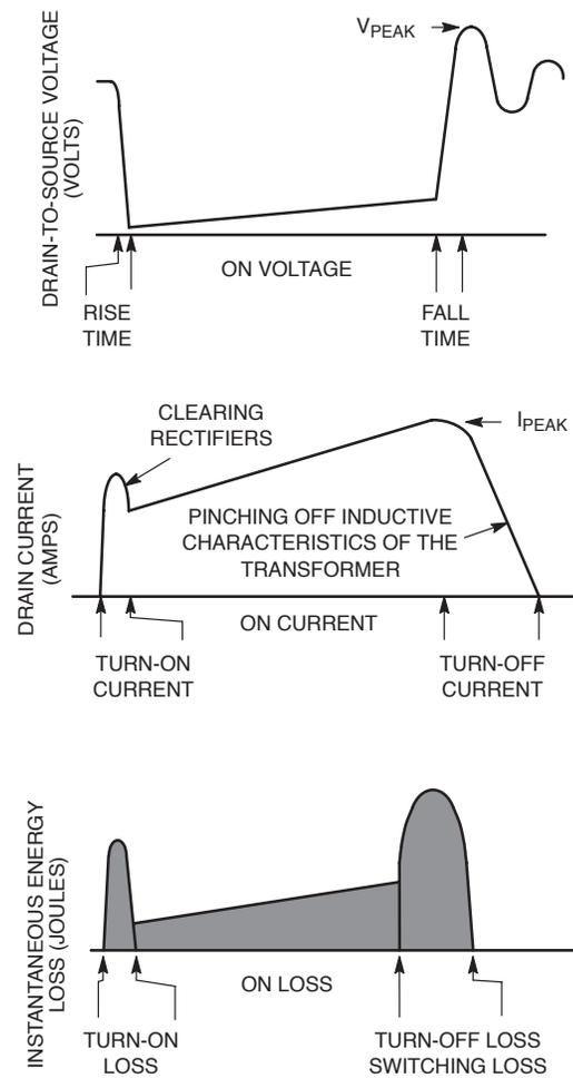
**Figure 24. Stresses and Losses within a Power MOSFET**
