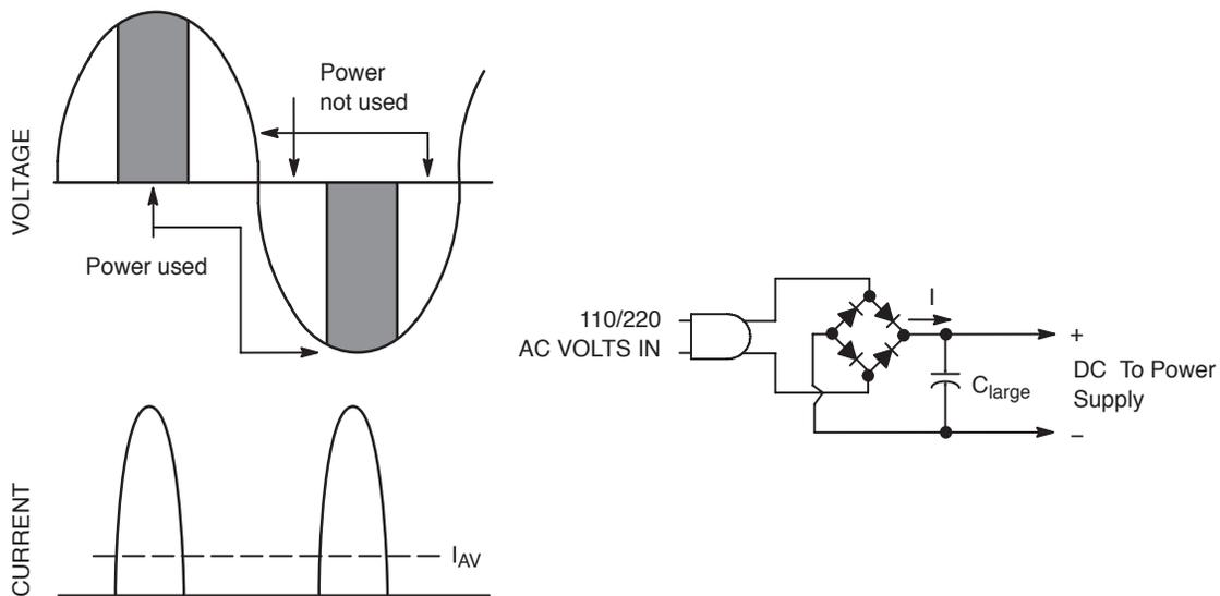
Figure 33. The Waveforms of a Capacitive Input Filter
