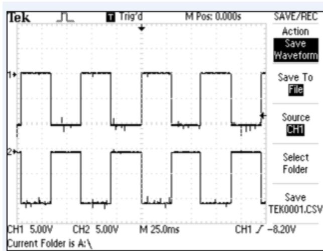
Carrier Signals which was supposed to give 16KHz:
