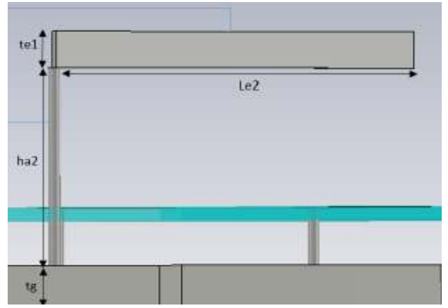
Fig. 6 Geometry of the low frequency element.
