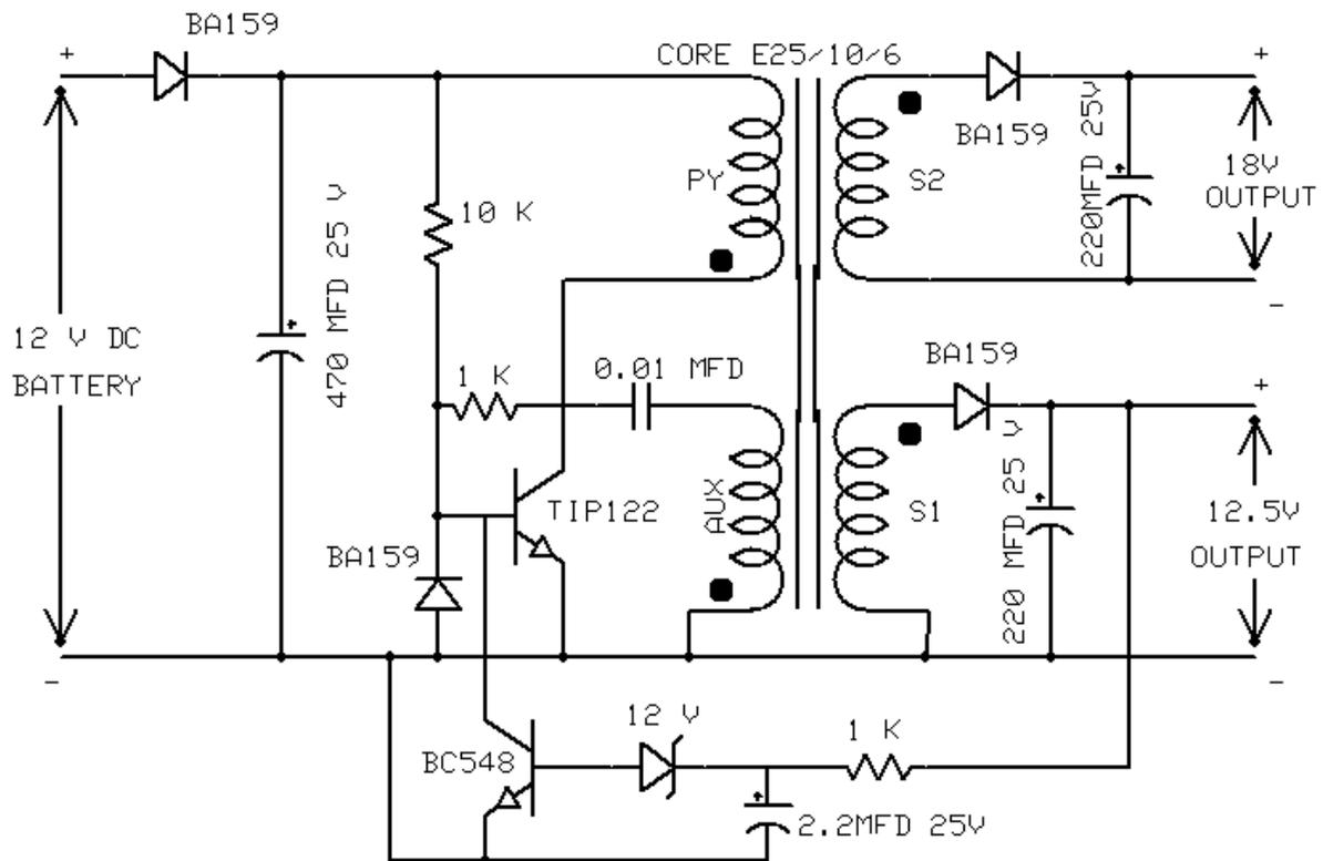
Peak Primary Current  $I_{\text{ppk}} = (2 \times P_o) / (\eta \times D_{\text{max}} \times V_{\text{min}})$
