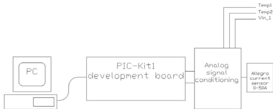
Figure 2, PIC processor based data acquisition system
