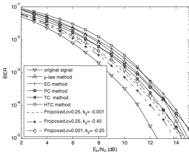
Fig. 8. BER performance of different transforms under the Rician fading channel for the OFDM system with  $N = 1024$  and QPSK modulation.
