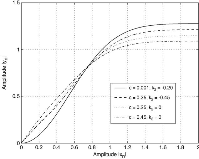
Fig. 1. Transfer curves of the proposed companding function.
