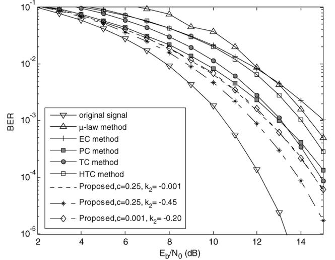
Fig. 7. BER performance of different transforms under an AWGN channel for the OFDM system with  $N = 1024$  and 16QAM modulation.
