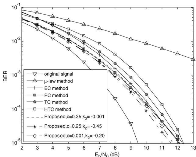
Fig. 9. BER performance of different transforms with SSPA ( $p = 2$ ) under an AWGN channel for the OFDM system with  $N = 1024$  and QPSK modulation.
