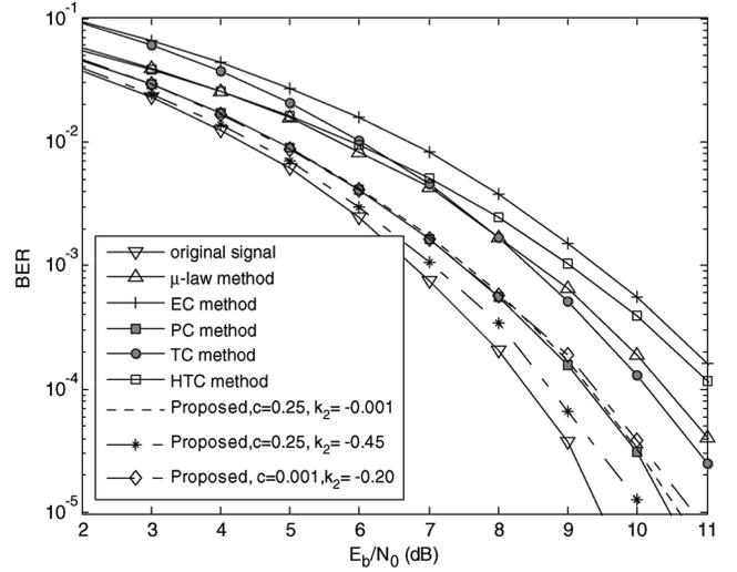
Fig. 6. BER performance of different transforms under an AWGN channel for the OFDM system with  $N = 1024$  and QPSK modulation.
