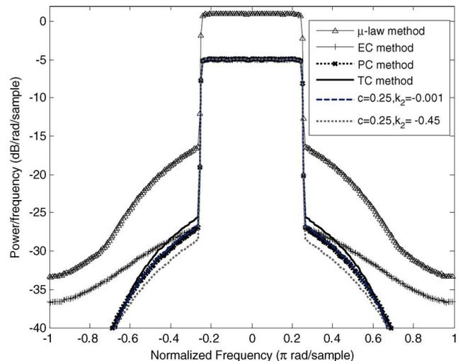
Fig. 10. Simulated PSDs of different transforms for the OFDM system with  $N = 1024$ , QPSK modulation, and oversampling ratio  $J = 4$ .
