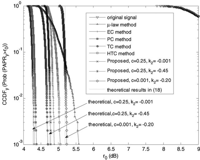
Fig. 5. PAPR reduction performance of different transforms for OFDM system with  $N = 1024$ , QPSK modulation, and oversampling ratio  $J = 4$ .
