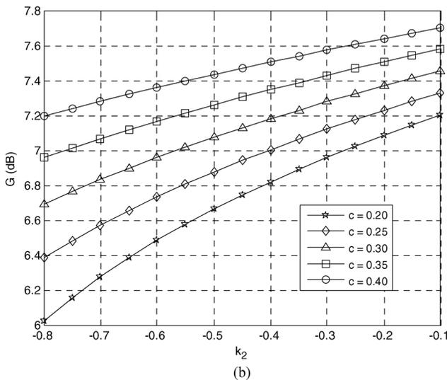
Fig. 2. Theoretical results of PAPR and G versus  $k_2$  of the proposed algorithm. (a) The ultimate PAPR of companded signals. (b) Transform gain G.
