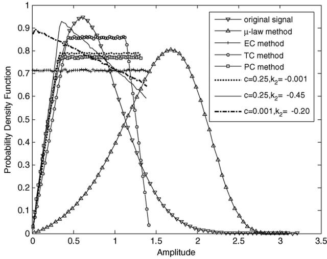
Fig. 4. The simulated PDFs of different transforms for OFDM system with  $N = 1024$  and QPSK modulation.
