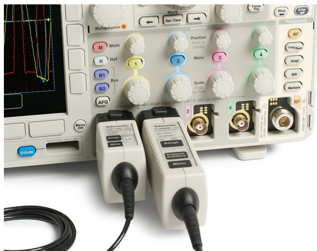
Figure 14. Voltage and current probes connected to oscilloscope with TekVPI interface.
