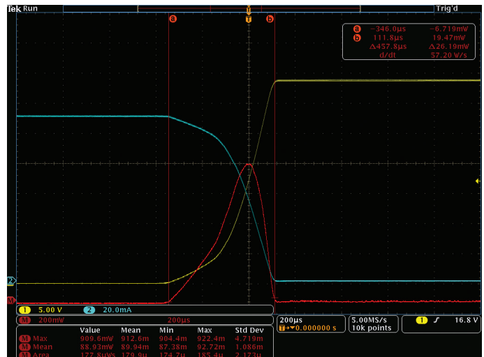
Figure 9d. After deskew procedure, mean power during switching is 89.94 mW, or 5.25% higher than before deskew.
