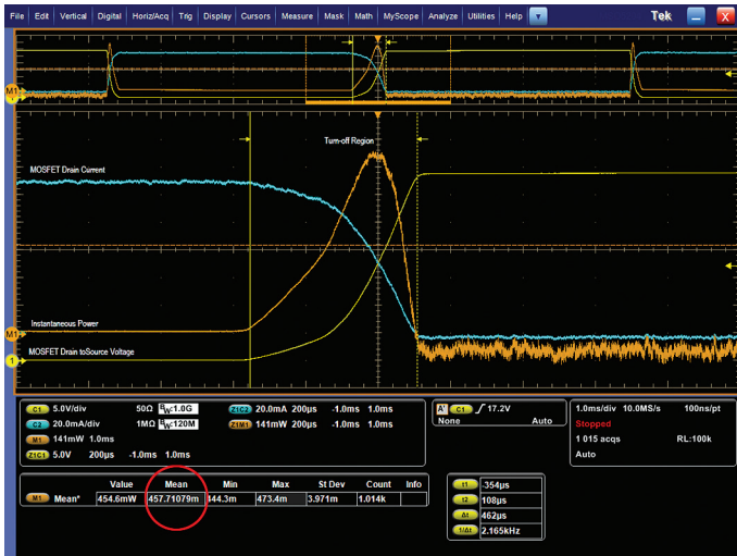
Figure 16. Switching loss measurement using oscilloscope's measurement toolset.
