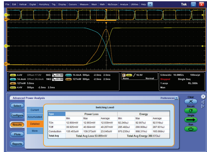
Figure 17. Automated measurement of switching loss using DPOPWR.
