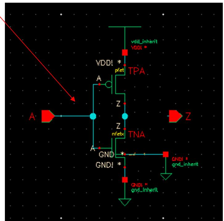
VDD! and GND! Inherited from the top level schematic.
